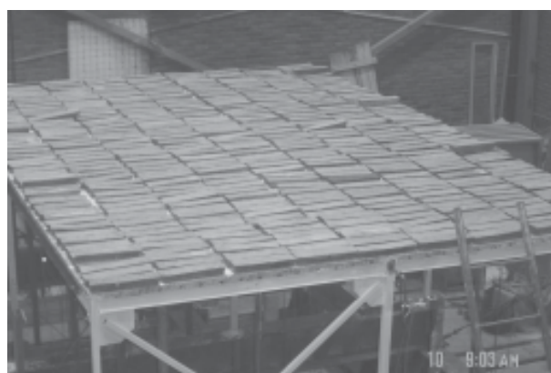
Figure 4. The gravity loading test.
