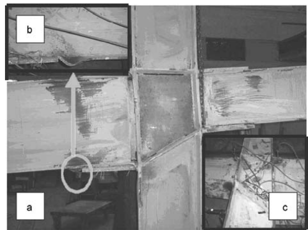
Figure 6. (a) Specimen U1-FUW1 erected after the experiment (rear view) (b) Deep beam flange buckling (front view) (c) view of fixed equipment for specimen U1-FUW1 during the test (front view).
