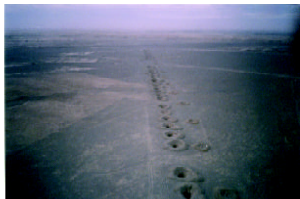
Figure 11. A Qanat trend near Bam city (The photo has been taken during pilot study by helicopter).
