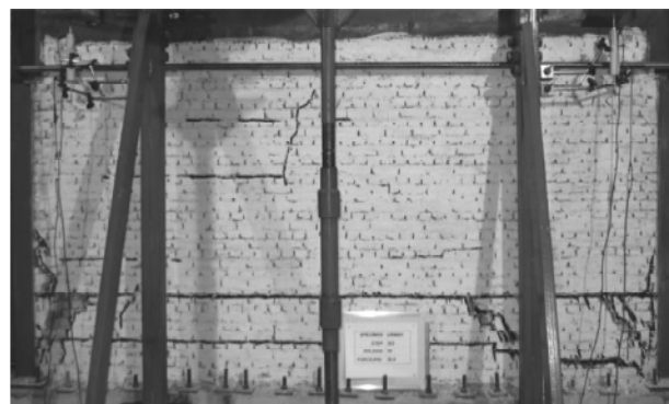
Figure 12. Crack pattern and hysteretic behavior of URMW-1.
