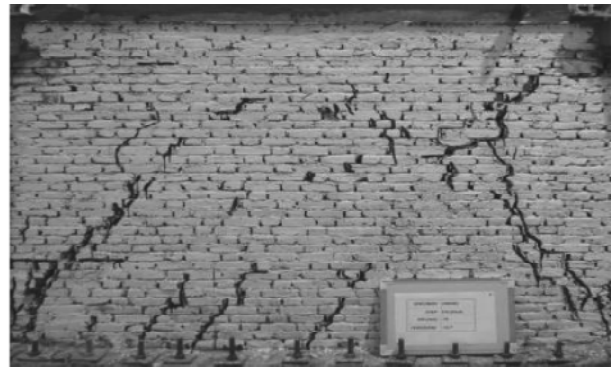
Figure 14. Crack pattern and hysteretic behavior of URMW-2.
