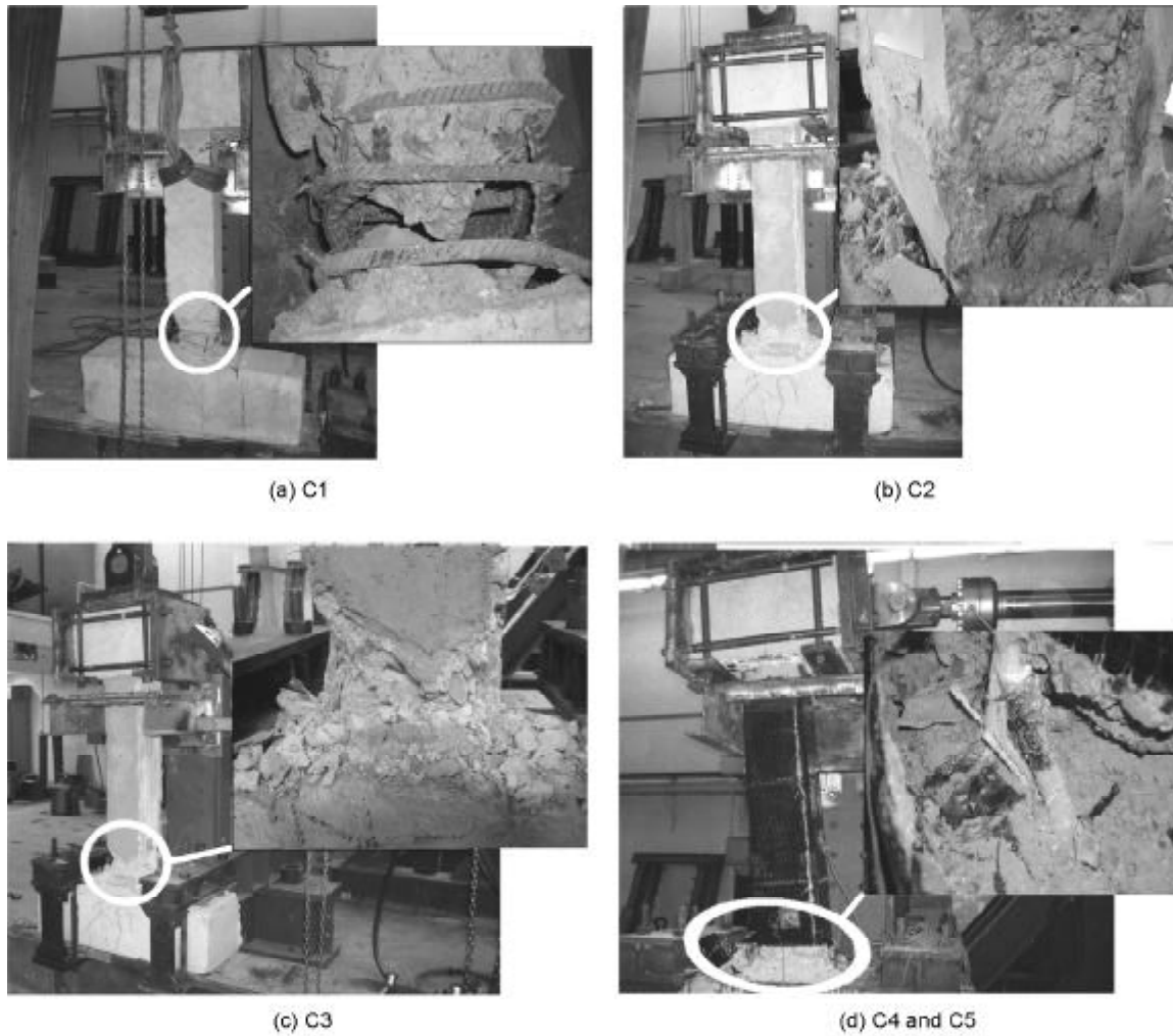
Figure 6. Test specimens at maximum lateral displacement.
