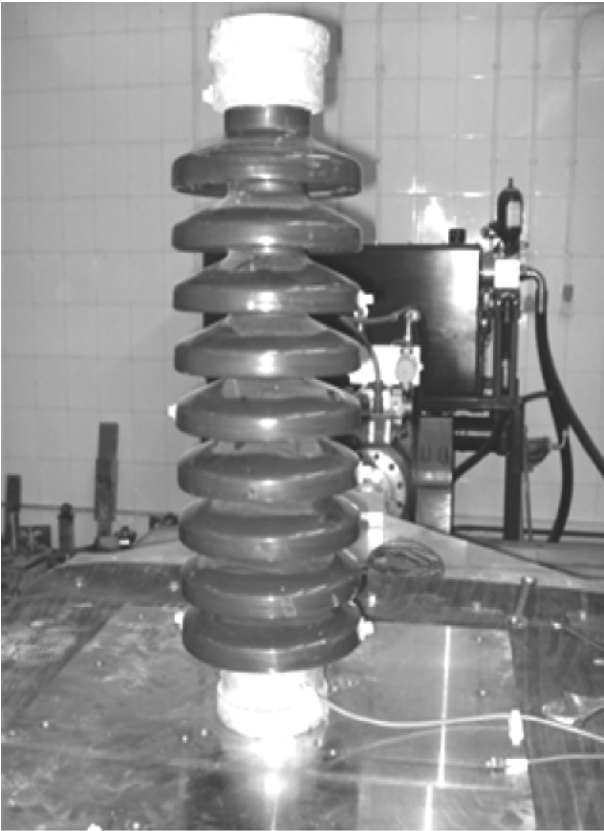
Figure 3. 63kV Post Insulator specimen.
