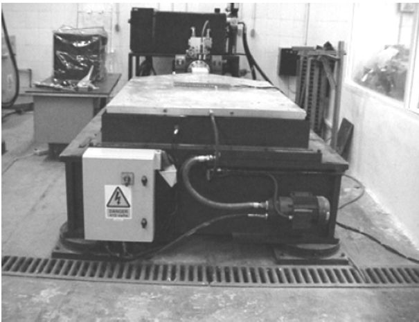
Figure 9. The IIEES shake table test facilities.
